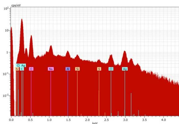
Fig. 7. Spectral analysis of the elements (SEM-EDS) of the silver layer with diamond nanoparticles deposited on aluminum substrate (sample 8\*)
